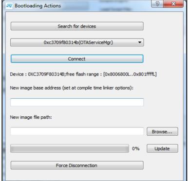
7 Once we have browsed to the application image built with the proper base address (0x8006800), we can press the "Update" button to start the OTA bootloading process. A progress bar will provide an indication of the time needed until process completion:
