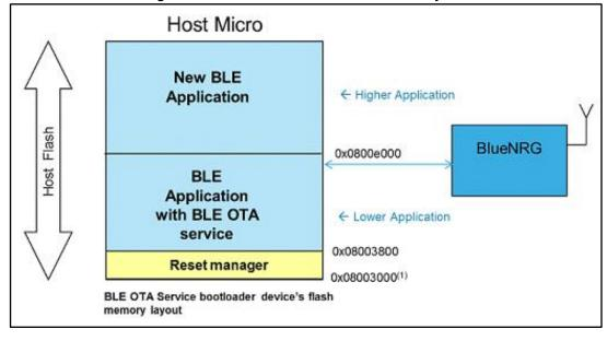
Figure 3: BLE OTA service bootloader Flash layout
