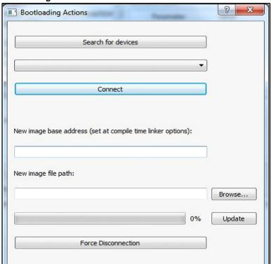
Figure 9: BlueNRG GUI: OTA bootloader window
