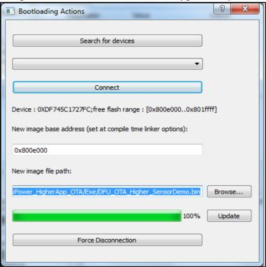
If we observe the slave board, we will find a change of color in the flashing LEDs notifying us that a new application is running. Tools such as the STM32 STLink utility can be used to check downloaded Flash memory regions on upgraded devices against the image within the selected binary files. After disconnection from the master, we can re-check the new version of the Sensor Demo functions against a "BlueNRG app for smartphones (IoS or Android)" as performed in step 2, optional items.
