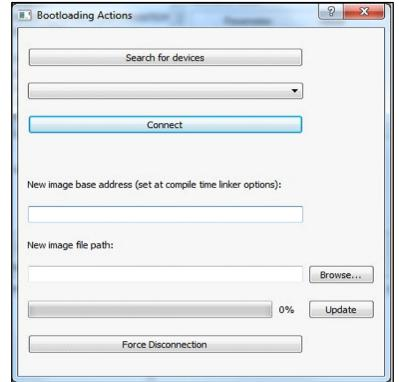
Figure 5: BlueNRG GUI: OTA Bootloader window
