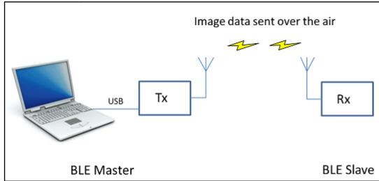
Figure 1: BlueNRG, BlueNRG-MS OTA master & slave devices
