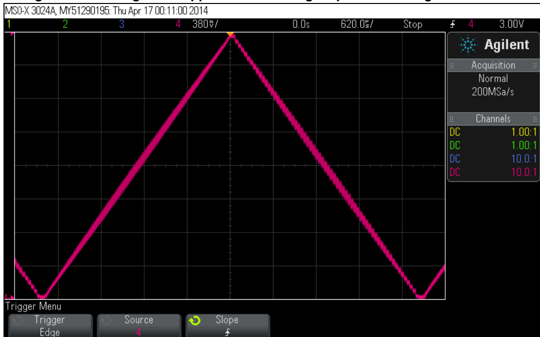
Figure 8. Dithering effect applied on the rising slope of the triangular waveform
