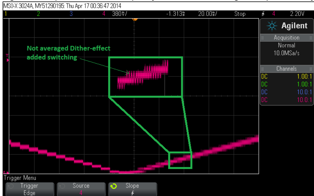
Figure 9. Low-pass filter cut-off frequency effect on the dithering technique efficiency
