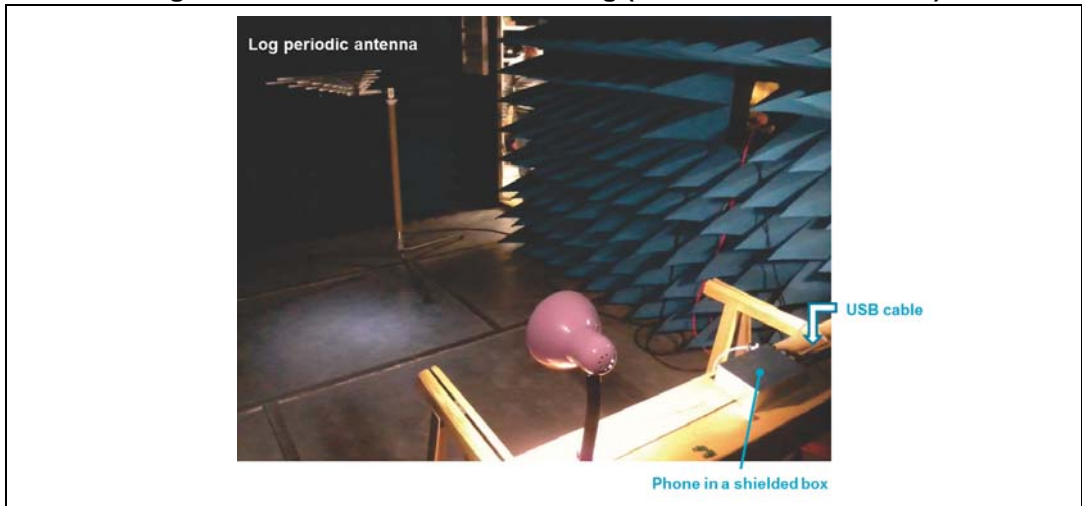
Figure 20. Radiated noise test setting (anechoic chamber view)
