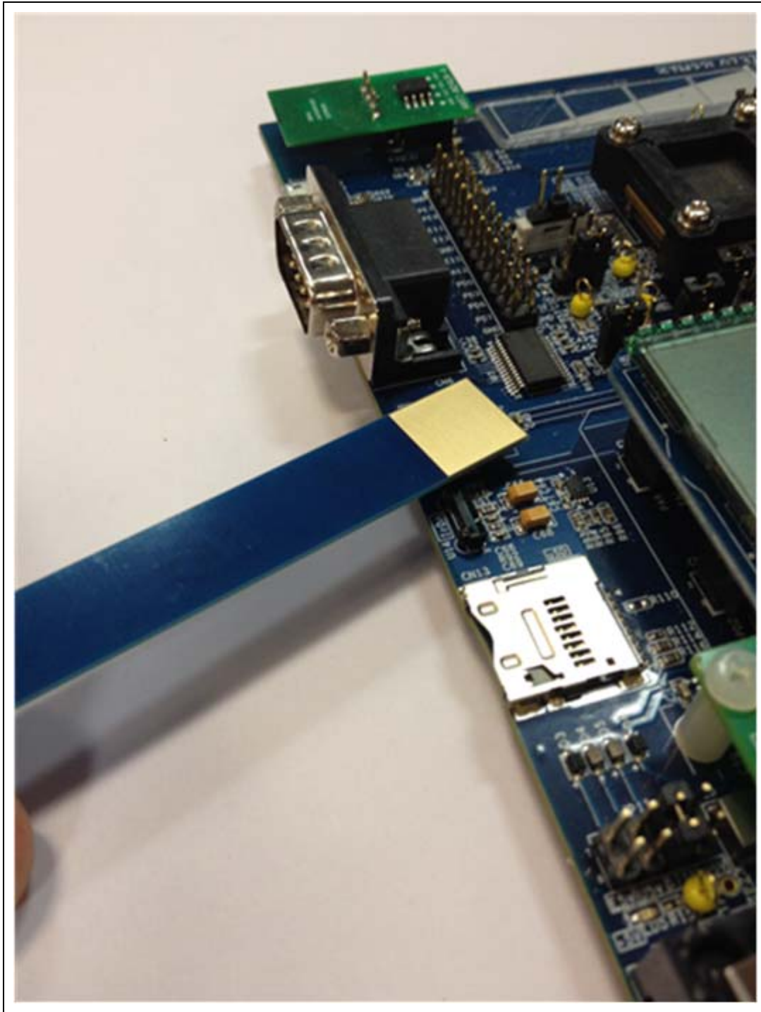
Figure 8. Using detection accessory board MB1199 with LC sensor metering
