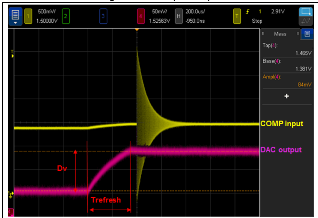
Figure 21. DAC output example
