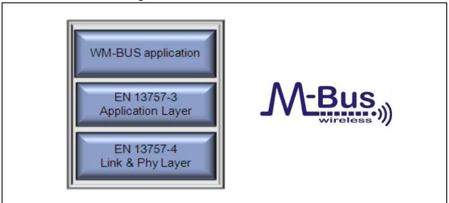
Figure 1: Basic Wireless M-Bus architecture
