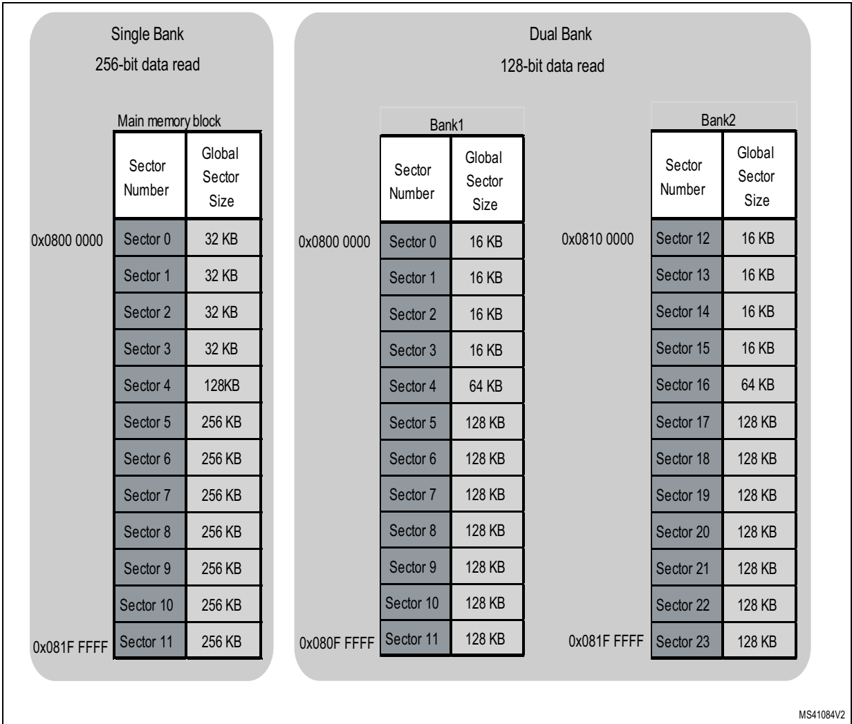
Figure 2. 2 Mbyte Flash memory organization
