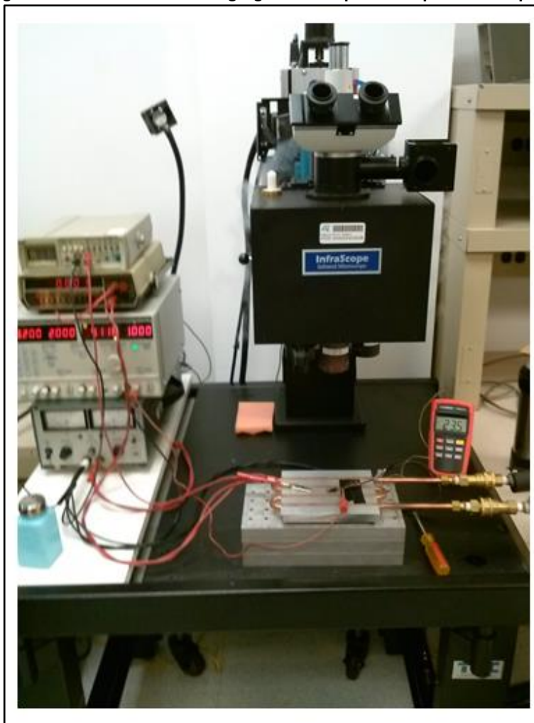
Figure 7: Infrared thermal imaging microscope with liquid-cooled plate
