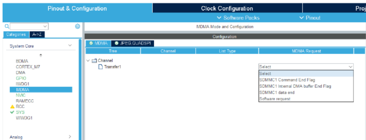
Figure 15. MDMA end of data configuration with STM32CubeMx
