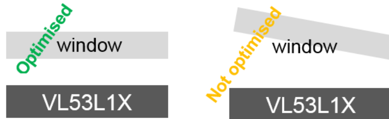
Figure 5. Example of cover glass tilt requirement with VL53L1X
