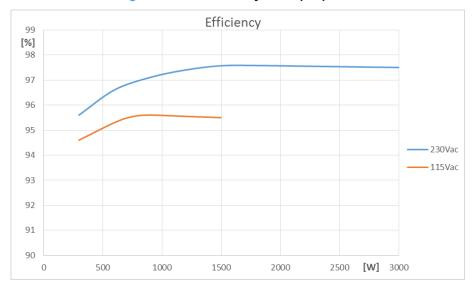
Figure 39. PFC efficiency vs output power
