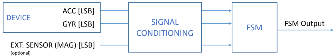
Figure 2. State machine in the LSM6DSOX
