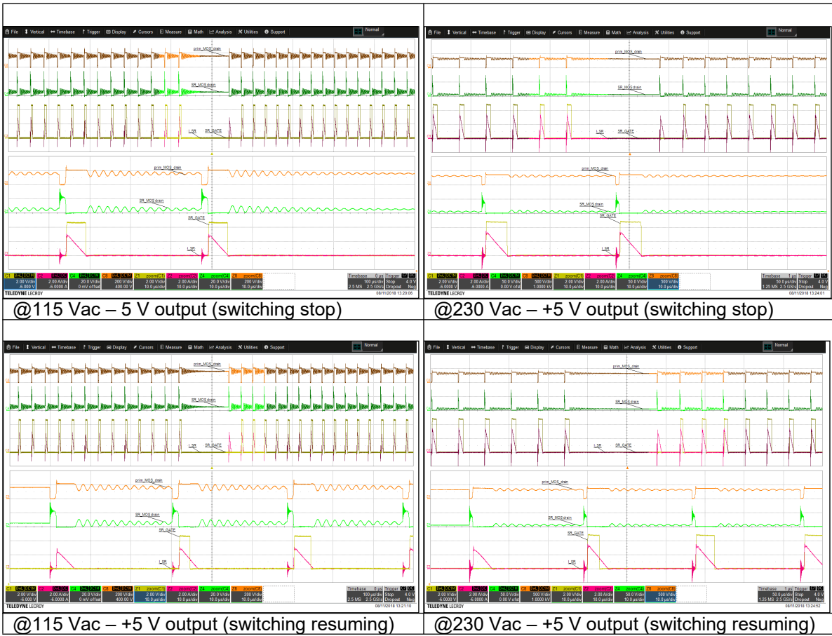
Figure 19. Typical burst-mode operation in no-load for +5 V output
