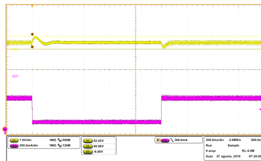
Figure 20. Load transients 230 V AC 75%-25%-75%
