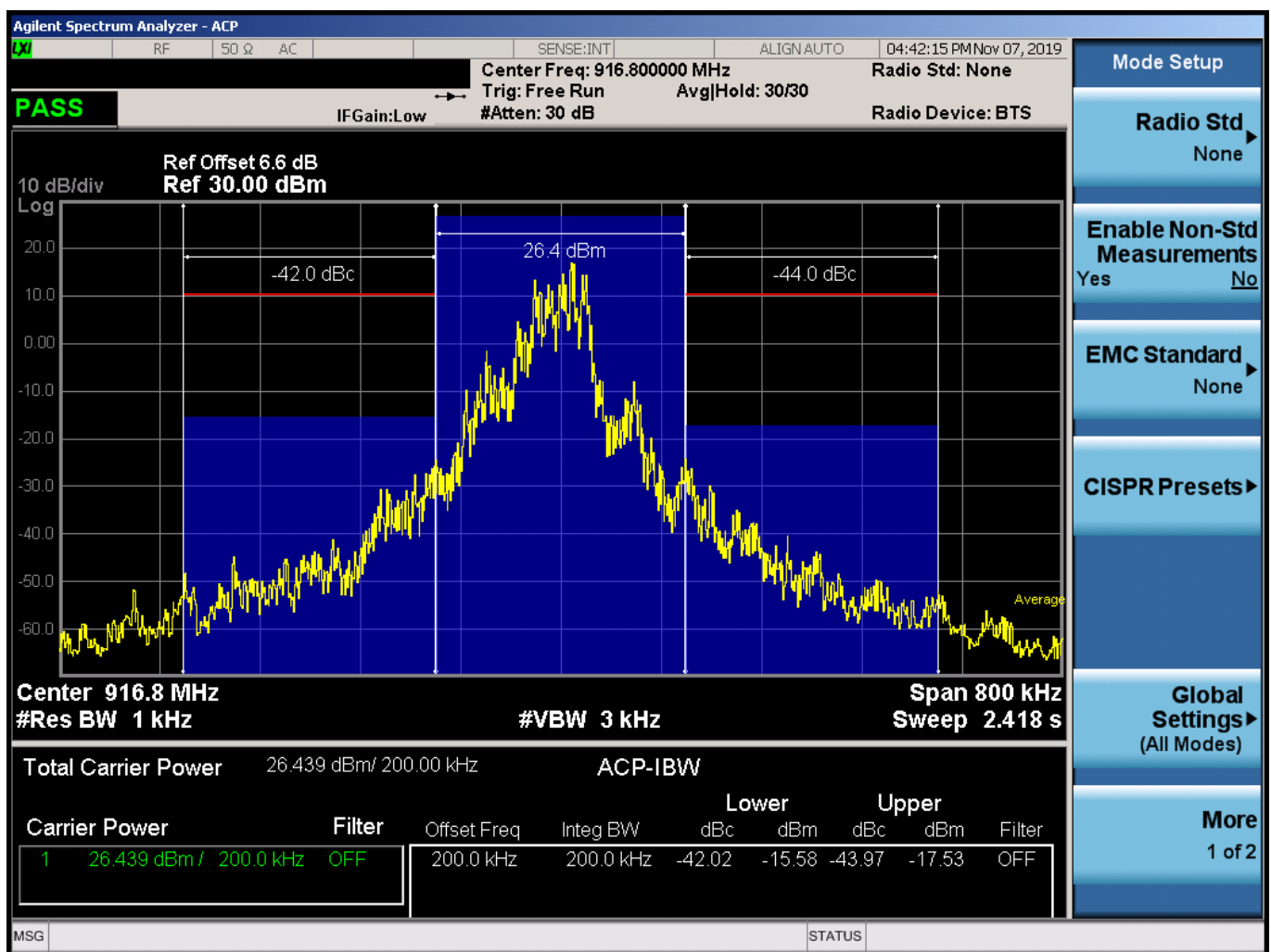
Figure 9. Adjacent channel leakage power results without SAW filter (TELEC – T240)
