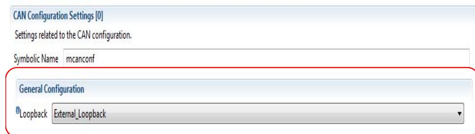
Figure 27. SPC5-Studio: CAN driver Loopback mode selection menu
