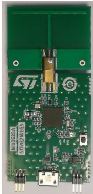
Figure 37. Monopole T-shaped antenna
