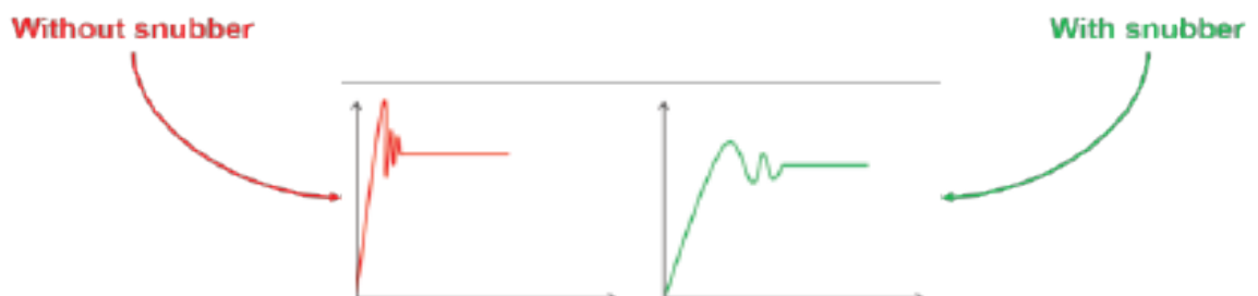
Figure 8. Impact of the snubber network on the slew rate at the drain of the MOSFETs
