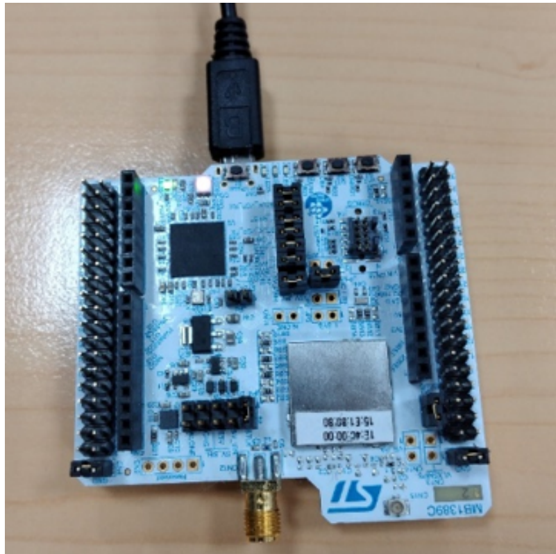
Figure 13. STM32WL55JC NUCLEO board in connected status
