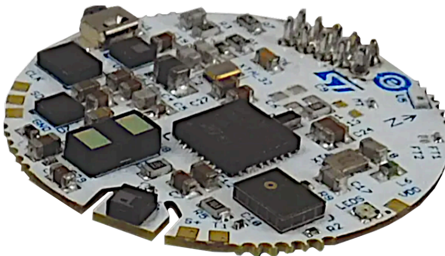
Figure 1. Bluetooth Mesh multi-sensor node supported by Sensor Server Model
