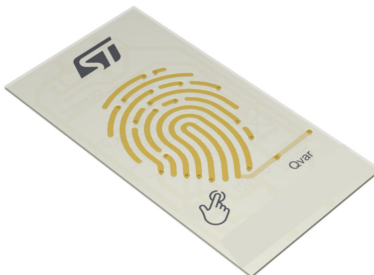
Figure 5. Example of a PCB electrode for touch detection (STEVAL-MKE002A)
