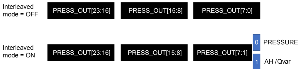
Figure 20. Analog hub / Qvar and pressure data tag
