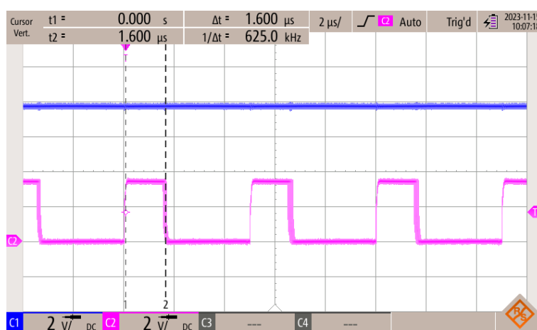
Figure 51. Output voltage and PWM for 0% load
