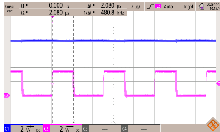
Figure 53. Output voltage and PWM for 100% load
