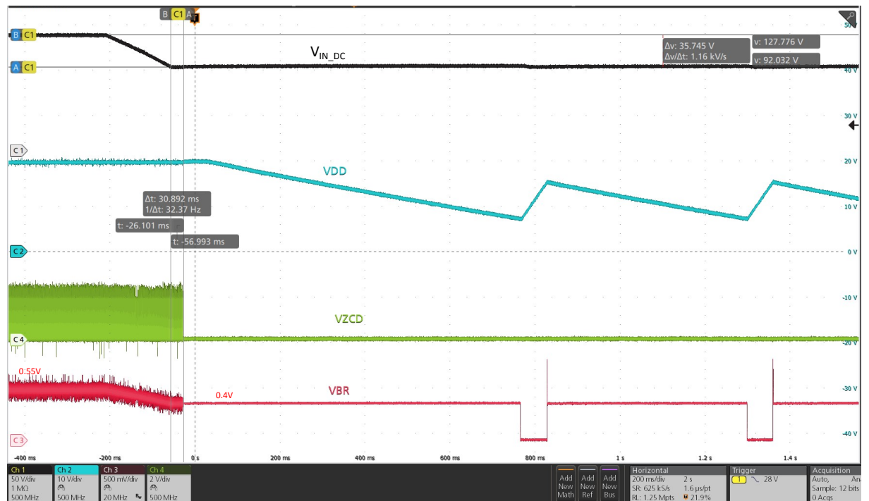
Figure 31. V_{IN} = 127 V_{DC} to 92 V_{DC} , brown-out triggered and IC stop
