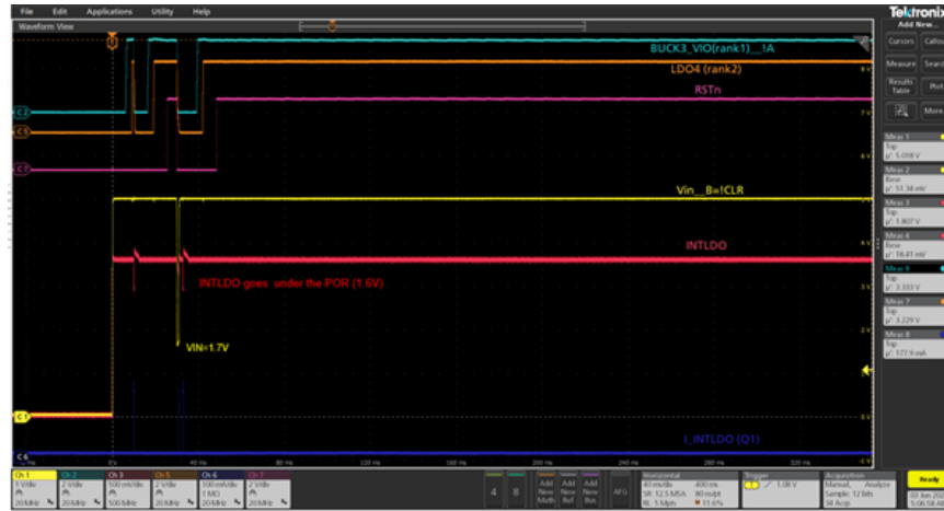
Figure 4. VIN brownout under the V_{INPOR\_Fall} after power-on (with the proposed circuit).
