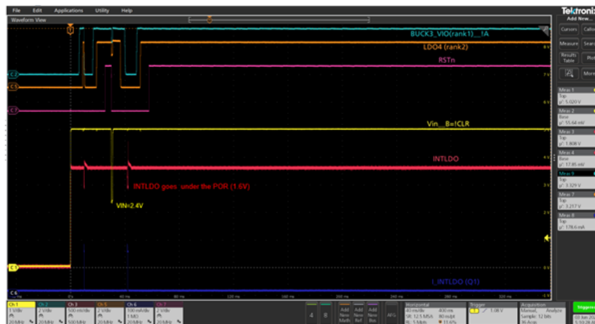
Figure 6. VIN brownout to V_{INPOR\_Fall} < VIN < V_{INOK\_Fall} after power-on (with the proposed circuit)
