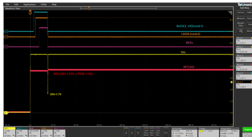
Figure 3. VIN brownout under the V_{\text{INPOR\_Fall}} after power-on (without the proposed circuit)
