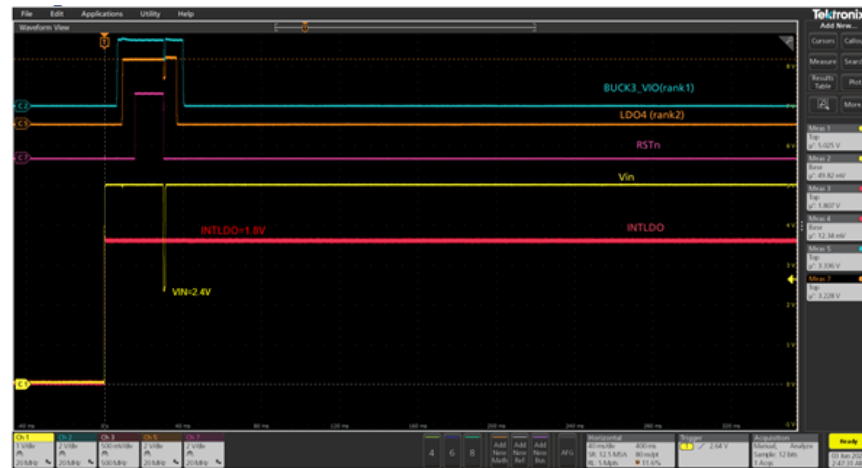
Figure 5. VIN brownout to V_{INPOR\_Fall} < VIN < V_{INOK\_Fall} after power-on (without the proposed circuit)
