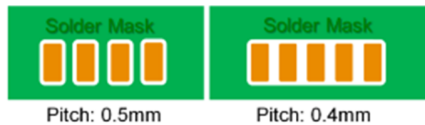
Figure 11. Solder mask opening for perimeter lands with pitch 0.5 mm and 0.4 mm
