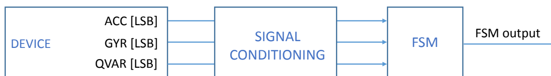
Figure 2. State machine in the LSM6DSV16BX
