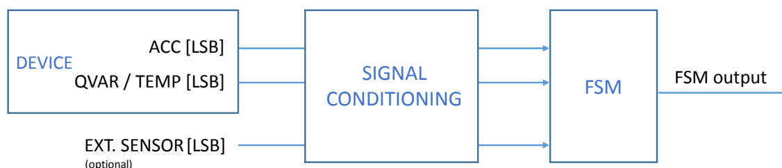
Figure 2. State machine in the LIS2DUXS12
