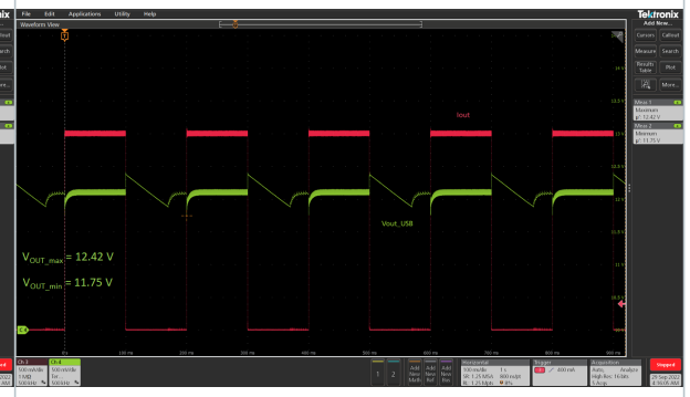
Figure 38. Dynamic step load ( V_{OUT} = 12\text{ V} , I_{OUT} from 0 to 3 A) at 230 V_{AC}
