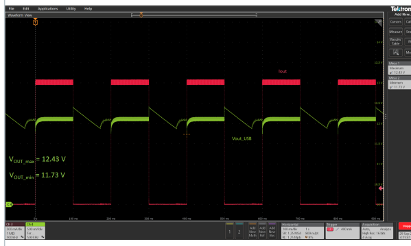
Figure 37. Dynamic step load ( V_{OUT} = 12\text{ V} , I_{OUT} from 0 to 3 A) at 115 V_{AC}
