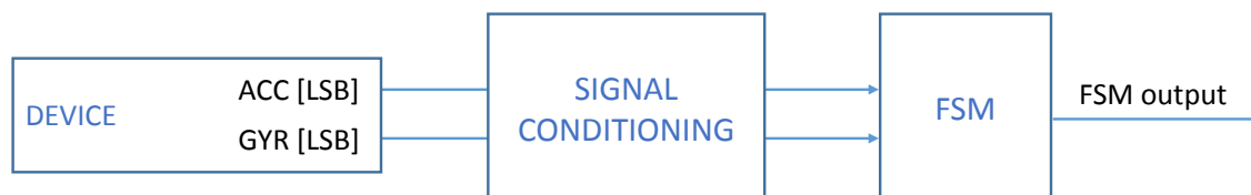
Figure 2. State machine in the ASM330LHB
