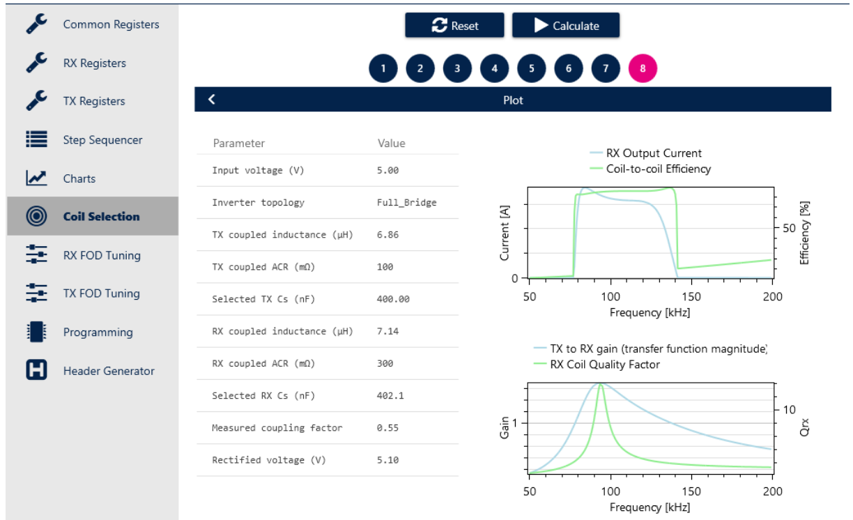
Figure 12. Output current and transfer function plots
