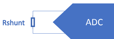
Figure 1. Schematic of the current measurement through a shunt resistor
