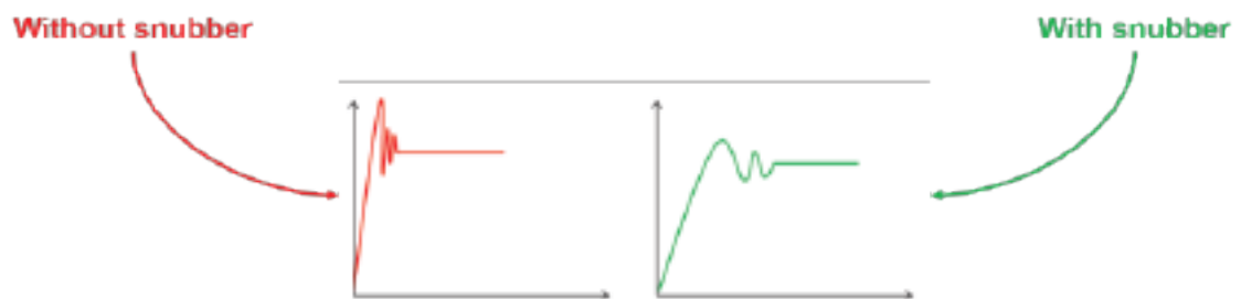
Figure 8. Impact of the snubber network on the slew rate at the drain of the MOSFETs
