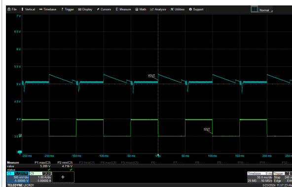
Figure 13. Dynamic load from 0% to 25% of 3.75 A, out 5 V, V IN =115 V AC
