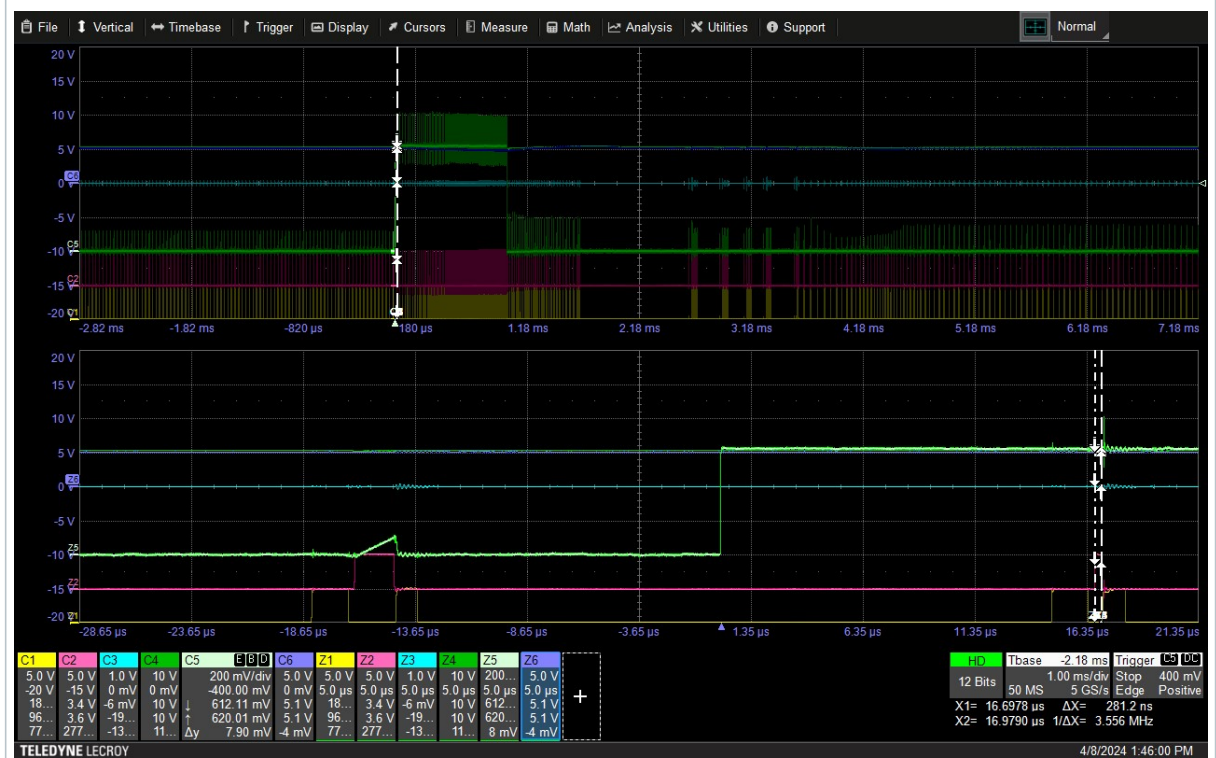
Figure 161. OC1 protection on primary side – 5 V output – 0.5 A load – 90 V AC input
