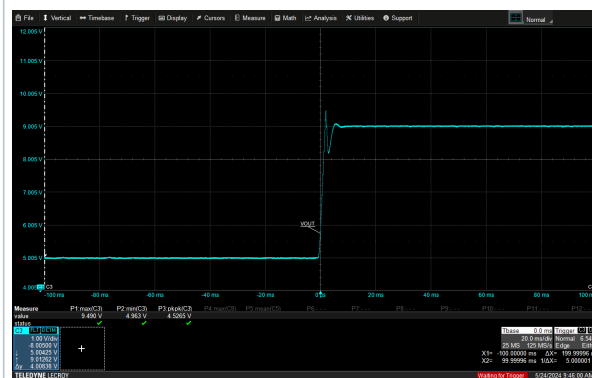
Figure 55. Voltage transition from 5 V to 9 V at 115 V AC - 3.75 A load
