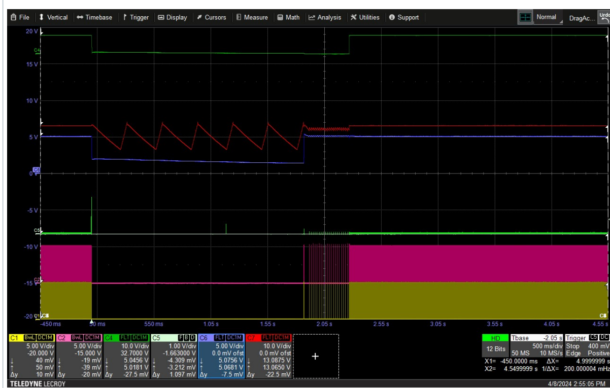
Figure 162. OC2 protection on primary side – 5 V output – 1 A load – 90 V AC input
