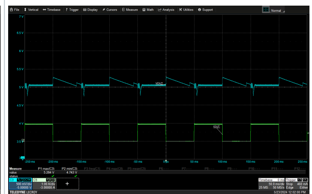
Figure 14. Dynamic load from 0% to 25% of 3.75 A, out 5 V, V IN =230 V AC
