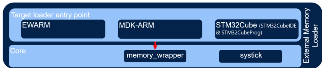
Figure 5. Architecture of external memory loader
