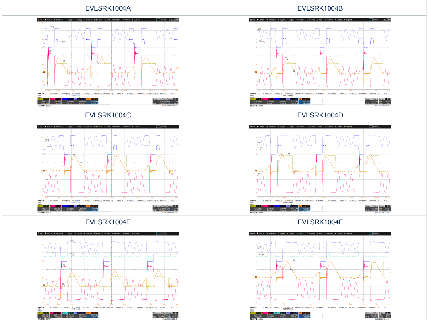
Figure 18. Key signals waveforms of EVLSRK1004 in LS mode on 65 W ACF @230 Vac V_{out}=20\text{ V} I_{out}=1.5\text{ A}
