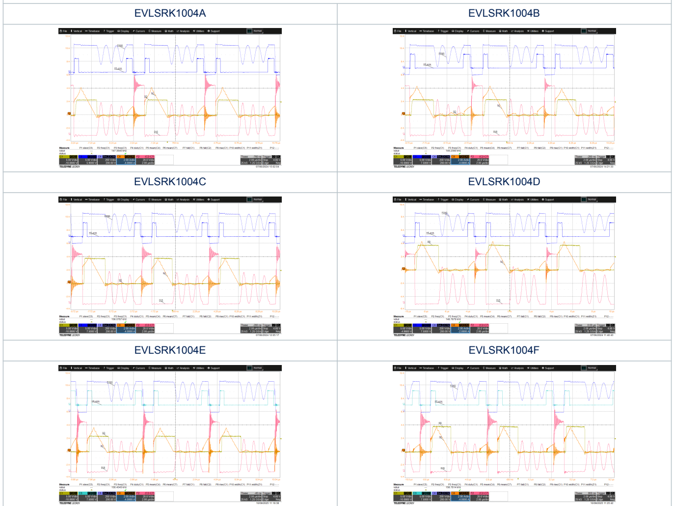
Figure 22. Key signals waveforms of EVLSRK1004 in HS mode on 65 W ACF @230 Vac V_{out}=20\text{ V} I_{out}=1.5\text{ A}
