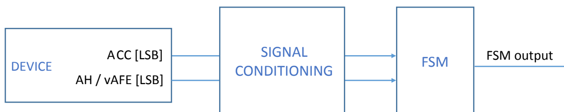
Figure 2. State machine in the ST1VAFE3BX
