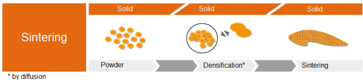
Figure 6. Basic schematic of the sintering process
