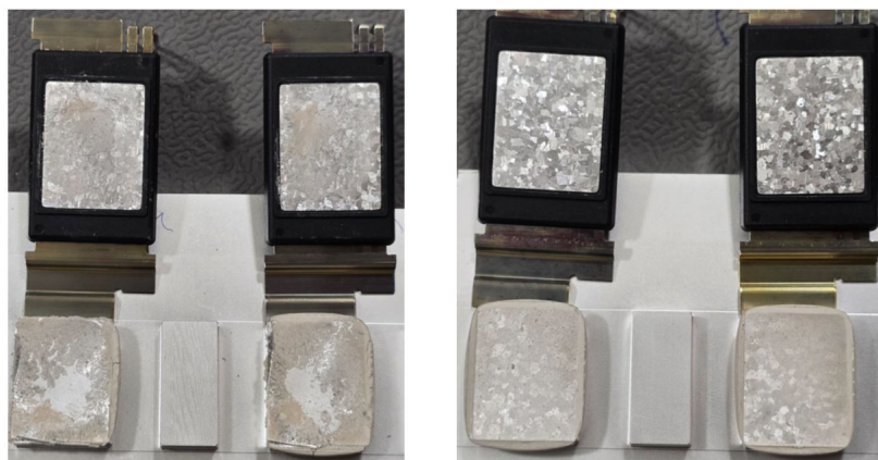
Figure 13. Example of cohesive (good) adhesion, on the left, and bad (adhesive) on the right
