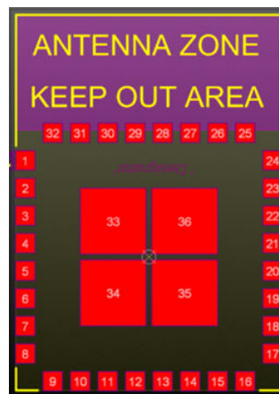
Figure 8. ST67W611M1 VIAs GND PAD
