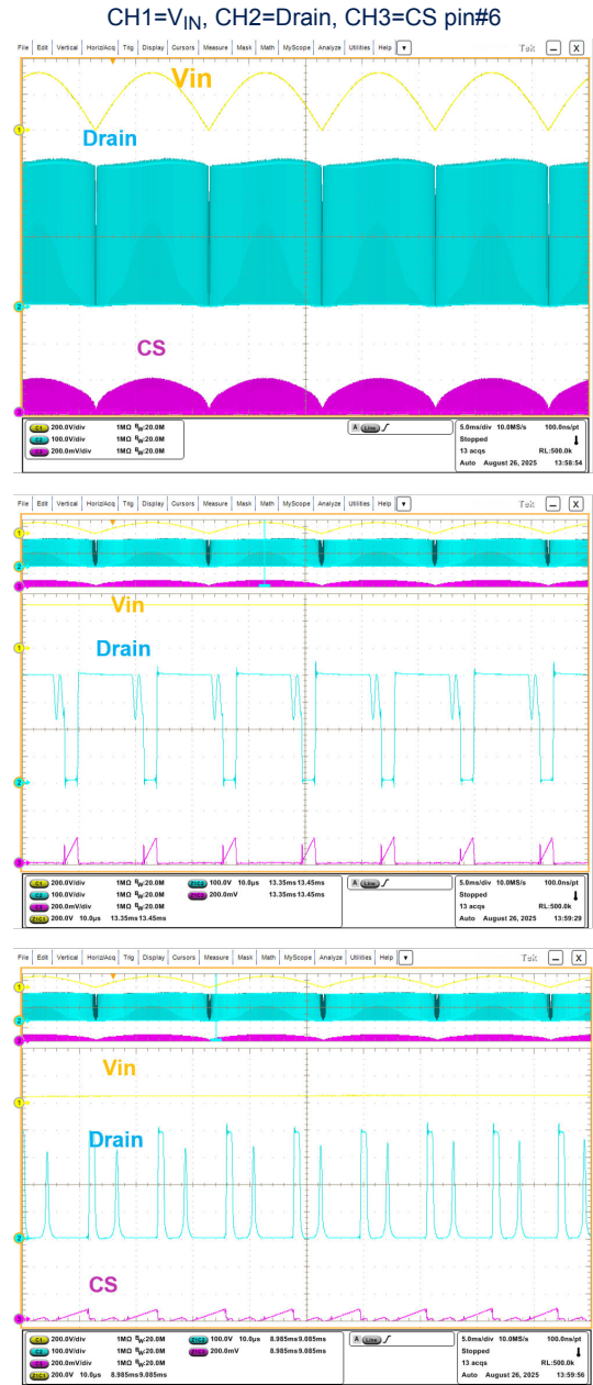
Figure 30. Steady-state – Valley turn-on at full load (230 Vac)
