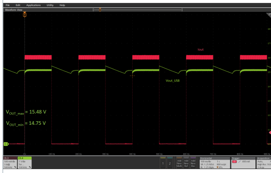
Figure 39. Dynamic step load ( V_{OUT} = 15\text{ V} , I_{OUT} from 0 to 3 A) at 115 V AC
