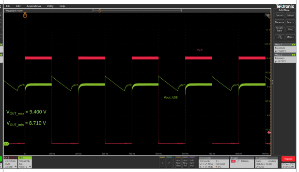
Figure 36. Dynamic step load ( V_{OUT} = 9 V, I_{OUT} from 0 to 3 A) at 230 V_{AC}
