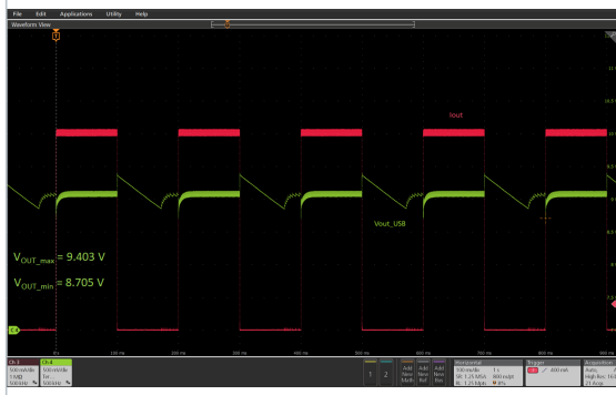
Figure 35. Dynamic step load ( V_{OUT} = 9 V, I_{OUT} from 0 to 3 A) at 115 V_{AC}
