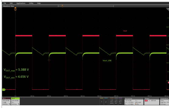
Figure 33. Dynamic step load ( V_{OUT} = 5 V, I_{OUT} from 0 to 3 A) at 115 V_{AC}
