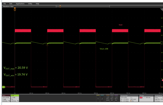
Figure 41. Dynamic step load ( V_{OUT} = 20\text{ V} , I_{OUT} from 0 to 3.25 A) at 115 V AC
