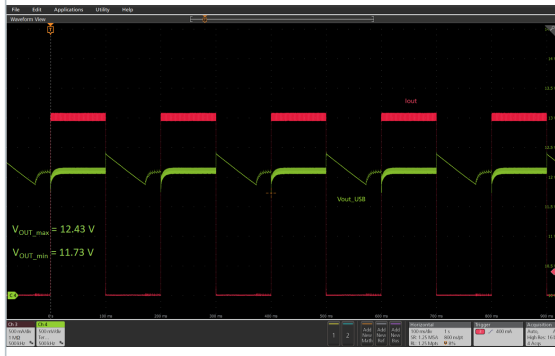
Figure 37. Dynamic step load ( V_{OUT} = 12\text{ V} , I_{OUT} from 0 to 3 A) at 115 V AC
