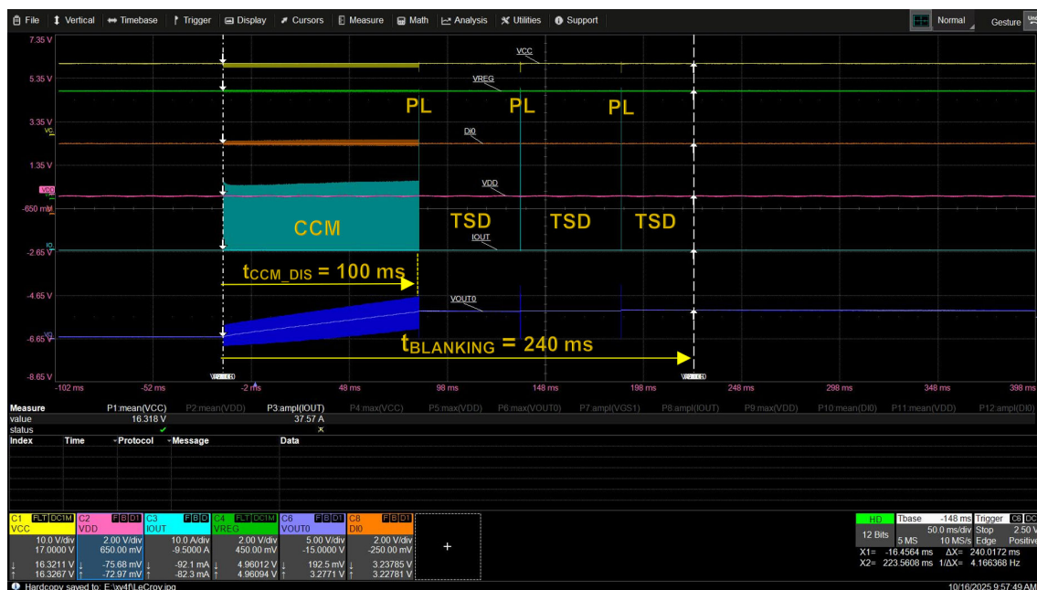
Figure 9. CCM charging with t_{CCM\_DIS} , expired, and TSD event occurred during power limitation with TSD events till Latch_OFF time expiration without charging completion
