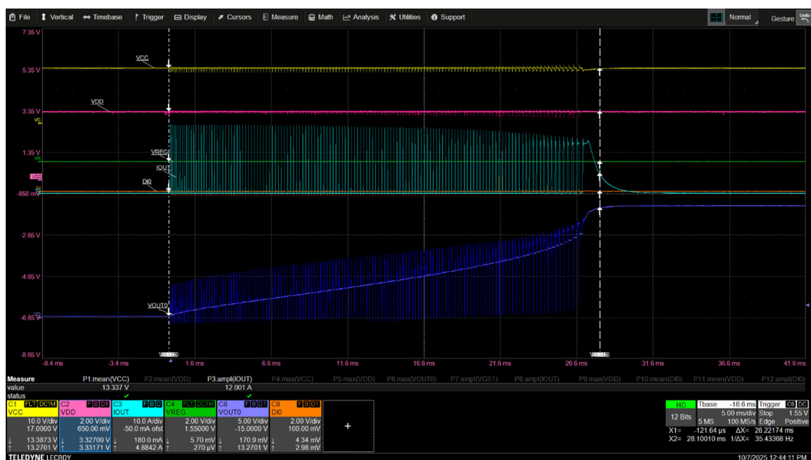
Figure 3. Capacity charging 13.5 V, T j = 25°C, C = 4.7 mF, ESR = 27 mΩ, T Saturation = 31 ms
