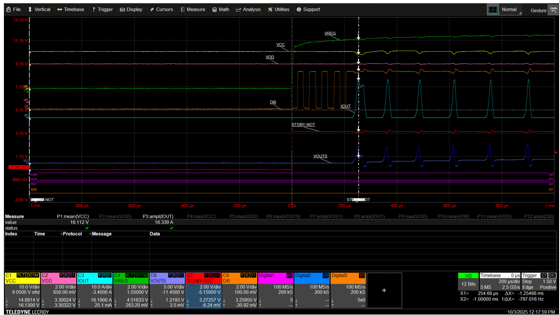
Figure 5. Rising edge particular of DI_0
