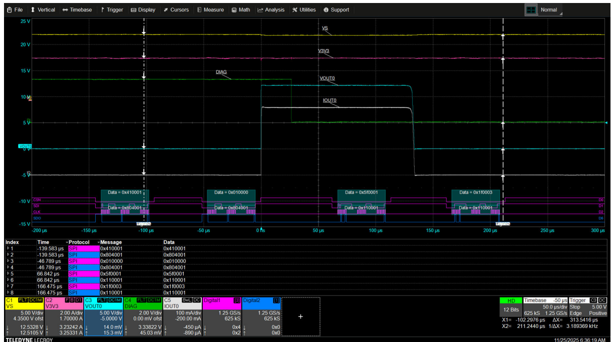
Figure 3. Device state transition (Normal to Fail-safe mode) and OUT 0 shut-down
