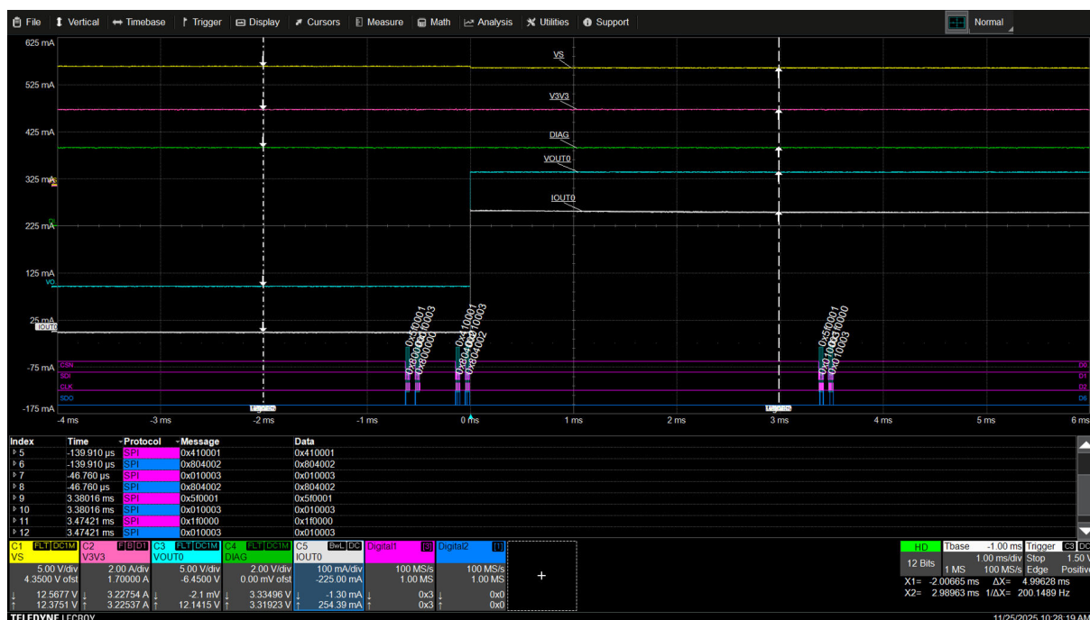
Figure 6. Device state transition (Normal to Fail-safe mode) without OUT 0 shut-down
