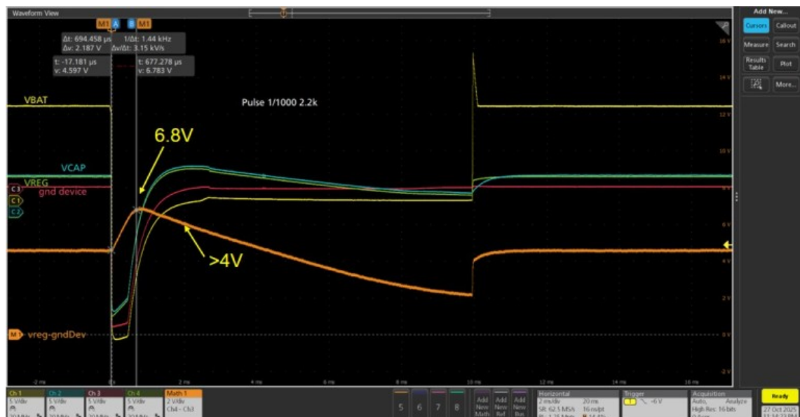
Figure 12. V_{REG} overvoltage during ISO 7637-2 pulse 1 with a 2.2 k \Omega series resistor on the NPN collector.
