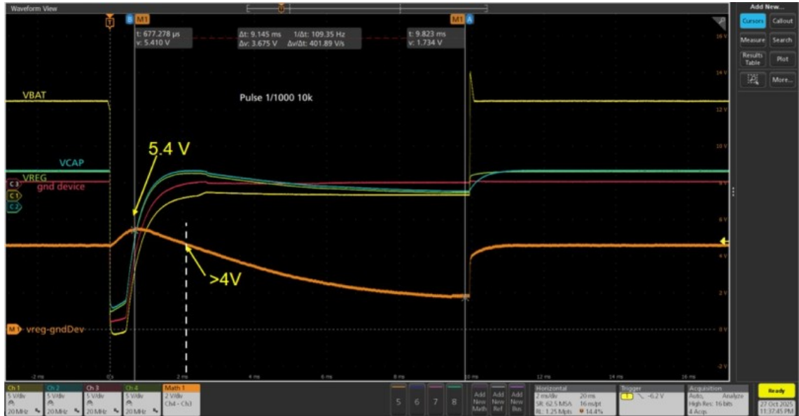
Figure 13. V REG overvoltage during ISO 7637-2 pulse 1 with a 10 kΩ series resistor on the NPN collector
