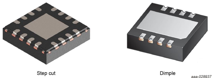
Figure 5. Wettable flank (WF) features of QFN/SON terminal ends
