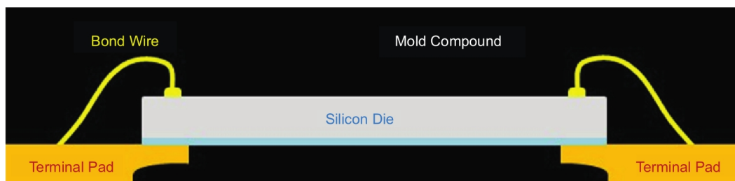
Figure 2. Chip-on-lead (COL) package design
