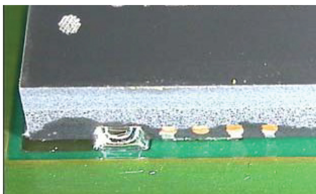
Shorts and Bridging on Perimeter Pads (Side View)
