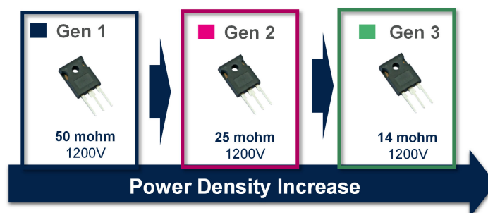
Figure 3. Technological enhancement from gen.1 to gen.3 for power density of the same package
