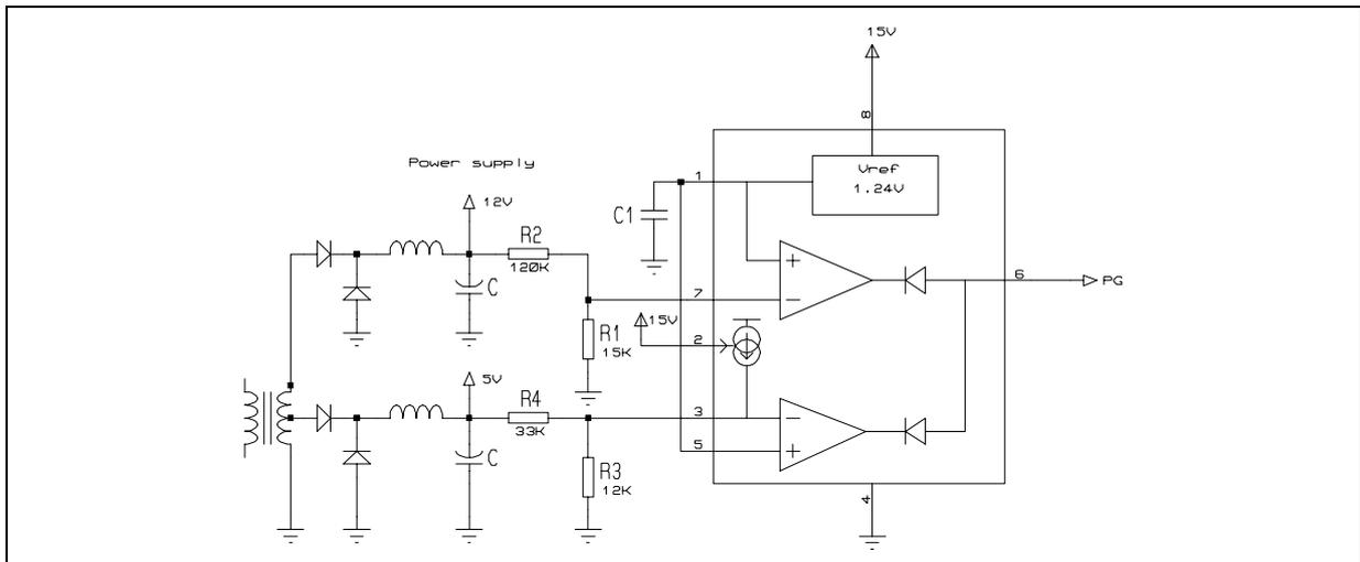
Inverting input (7) and non inverting input (5) are respectively used for overvoltage and undervoltage detection.
