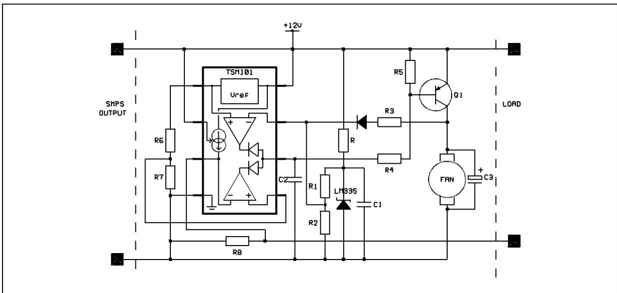
Let us assume that TSM101 is used as a thermostat for an application which has a maximum consumption of 10A and requires air flow starting at a current consumption of 2A.
