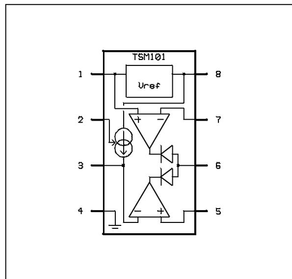
Figure 2 : Basic Thermostat Function
