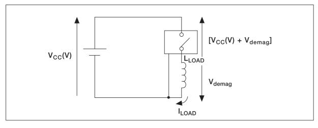
The source of the power MOSFET becomes more negative than the ground until it reaches the demagnetization voltage,  $V_{\text{demag.}}$ , of the specific device. In this condition the inductive load is demagnetized and its stored energy is dissipated in the power MOSFET according to the equation shown below:
