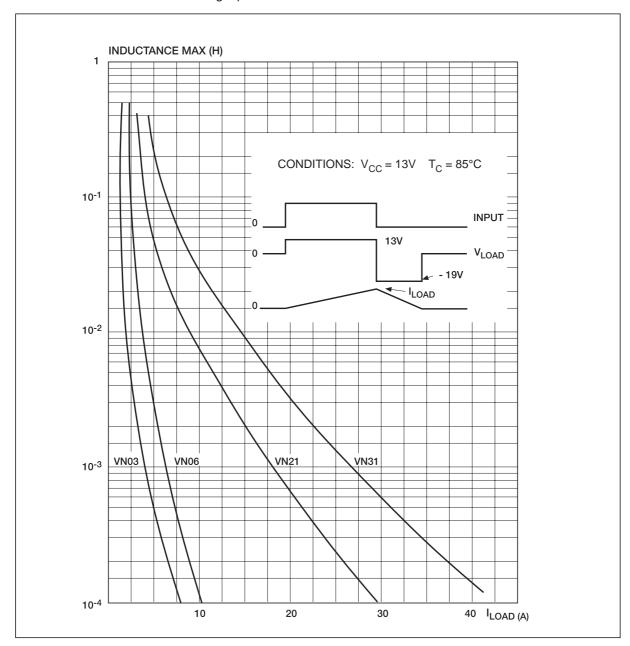
**Figure 8**: Max inductance which produces a temperature of 160°C at turn off with Vcc = 13V. The values are for a single pulse with Tc = 85°C
