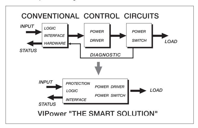
Vertical intelligent power, (VIPower ™) an SGS-THOMSON Microelectronics patented technology, established over 7 years ago, uses a fabrication process which allows the integration of complete digital and/or analog control circuits driving a vertical
