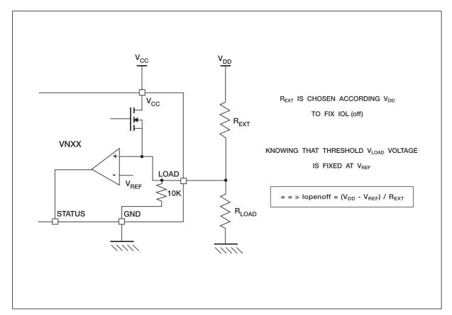
Open load detection is possible in the off-state in the VN21 family and it conforms to the I.S.O. norms for automotive applications. If an open load condition is detected the status flag goes low. Should an external supply be applied to the load (output pin) or the device is externally short circuited, the off-state open load detection can detect this "stuck-on" to  $V_{\rm CC}$  condition.
