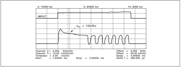
Even in this configuration, the device controls the di/dt. Figure 9 shows a start-up when there is a short circuited load driven by a VN05N. The initial peak current is 30A for this  $180m\Omega$  device.
