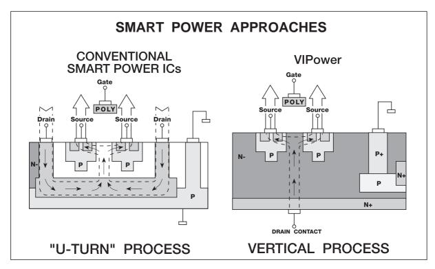
The VIPower technology M0 used for making these High Side Drivers produces a monolithic silicon chip which combines control and protection circuitry with a standard power MOSFET structure where the power stage current flows vertically through the silicon.
