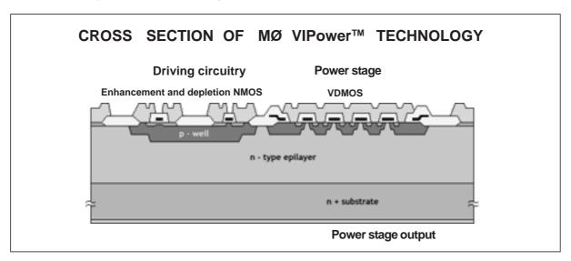
High Side Drivers, with their integrated extra features are power switches that can handle high currents and work up to about 40V supply voltage. They require only a simple TTL logic input and incorporate a fault condition status output. They can
