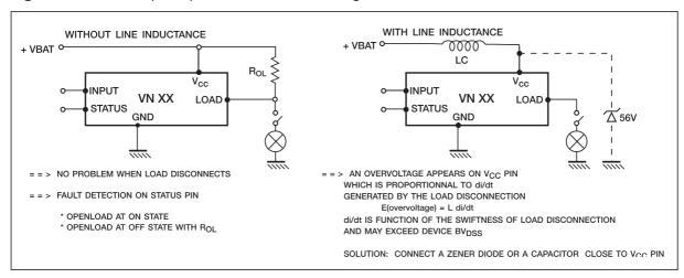
Figure 14c: Behaviour of a VN21 during a load disconnection
