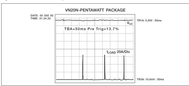
Figure 11: Automatic Thermal cycle in overload condition
