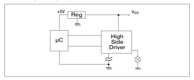
The second case, shown in fig. 15b, is when both the GND pins of the High Side Driver and of the µC are disconnected while the load is connected to ground. In this situation the signal GND rises up to V<sub>CC</sub>. In the I.S.O. and industrial High Side Drivers nothing happens up to  $V_{CC}$ <18V and the diagnostic output remains in high
