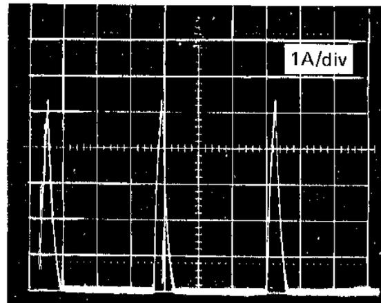
Current at Pin 2 when the Output is Short Circuited.
