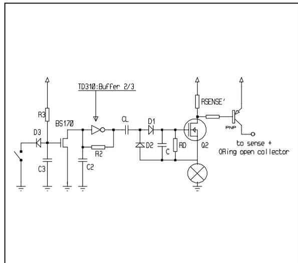
Figure 6 shows the ready to use applications (blinker and timing functions) described above where both applications are short circuit protected by the same sense comparator.
